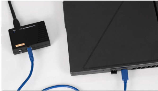
Figure 1: Plug the USB-A connector end of the provided cable bundle into the Super Speed Hub.
